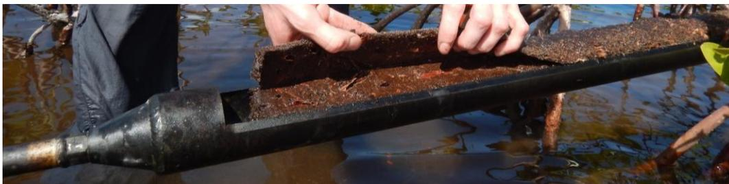
Figure 2. Image of an open-faced gouge corer with a mangrove peat core. The top portion of the core is being removed before the subsamples are collected (Photo: C. Beers).
